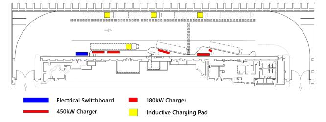
Figure 19: Commerce Street Station Electric Bus Charging Layout
