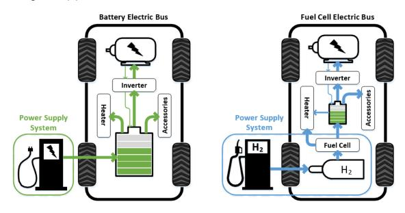
Figure 1: Battery Electric and Fuel Cell Bus Technologies
