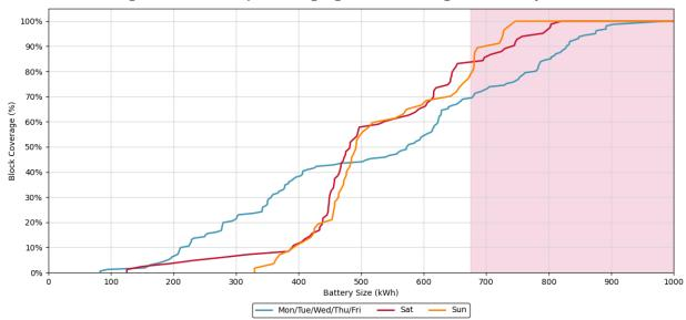
Figure 43: BEB Depot Charging Block Coverage vs. Battery Size
