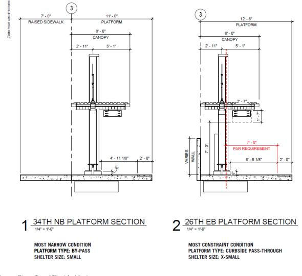
Figure 14 Curbside Pass-Through and Bypass Station Cross Sections
