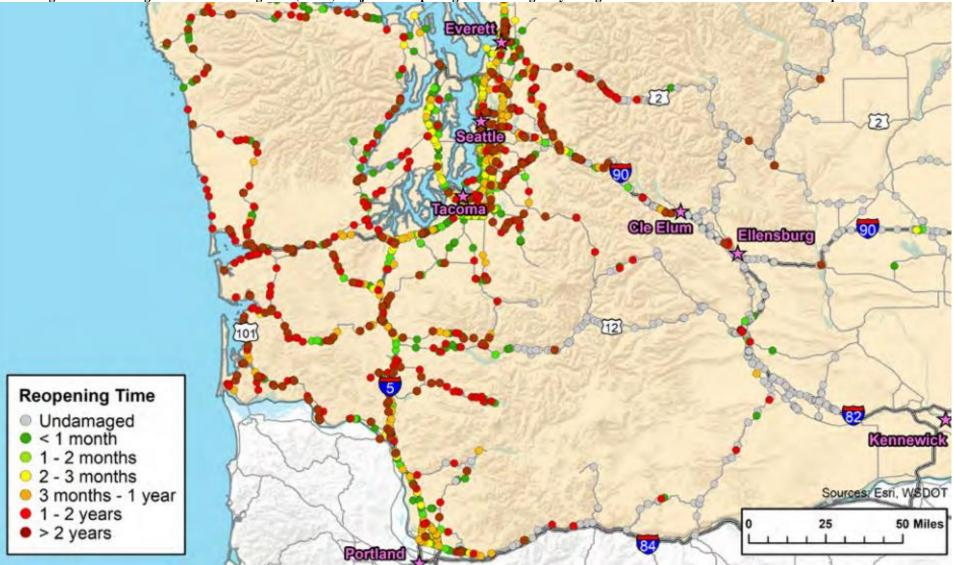
Figure 4.2 – 6 Bridge Seismic Screening Tool (BSST) Projected Reopening Times of Highway Bridges in WA After the CSZ Scenario Earthquake<sup>41</sup>
