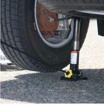
Raise the vehicle until tire is completely off of the ground.
