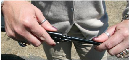
Assemble jack handle sections together and lock into place.
