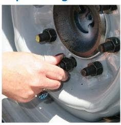
Thread the lug nuts onto the lug bolts with beveled face toward the wheel.
