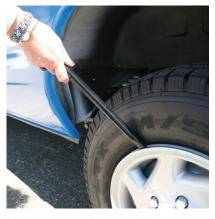
• Insert tapered end of lug wrench behind wheel cover and twist off.
