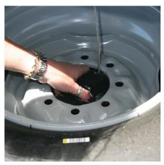
• Turn jack handle counterclockwise until the cable is slack and the tire can be slid from under the vehicle.
