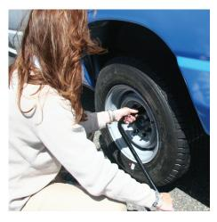
• Use lug nut wrench, turning clockwise, to screw lug nuts snugly against the wheel.
