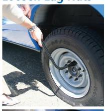
Using lug wrench and turning counterclockwise, loosen wheel lug nuts
