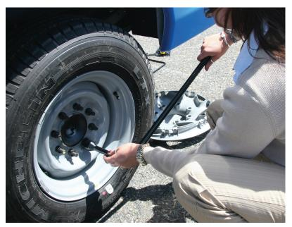
Finish removing lug nuts with the lug wrench.
