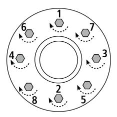
Remove the jack and fully tighten lug nuts clockwise with the lug wrench in the following pattern. Follow the order of the numbers.
