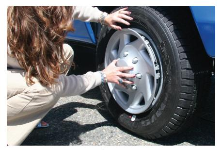
Install the wheel cover, if your van has one, making sure it is securely snapped into place.
