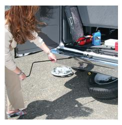
• Insert tip of the jack handle through the access hole and into the tube.
